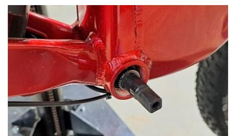
2. Once the right-side cup is removed, slide the B.B. set out from the right side of the bike and be careful not to damage the wire. Pull the B.B. set out with its wire attached and unplug it at the connection with the main wire harness as it comes out. You can now fully remove the B.B. set on that right side (only if needed by unthreading it counterclockwise).
