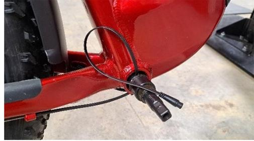
3. We advise not to touch the BB set unless it absolutely needs to be replaced. The tightening of the cups as simple maintenance needs to be done very carefully, and the left-side cup should never be tightened or undone without the B.B. set being removed half-way through the right side (disengaged from the left-side cup).
