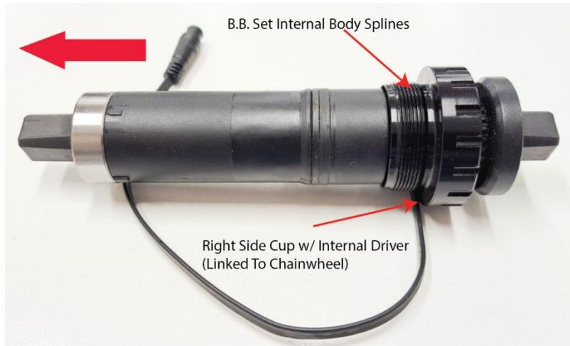
5. In some cases, if the B.B. set wire cannot be gently pulled / removed and its plug is not accessible through the B.B. shell, it will be necessary to remove the battery, the lower battery mount and the controller located beneath to access that wire and its plug for disconnection and re-installation.
