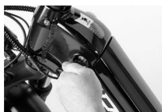
Lock battery in frame
