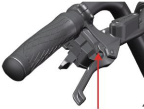
Fine adjustment bolt / 2mm Allen wrench
