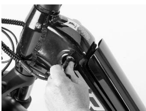
Unlock to push battery down
